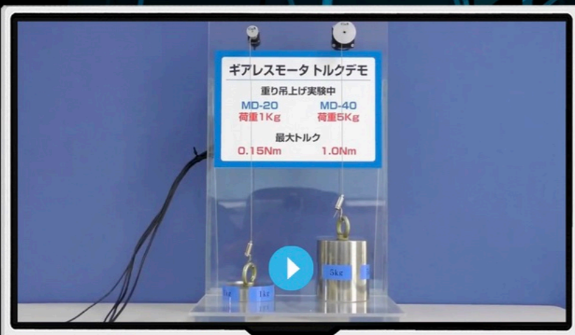
Video: Torque demonstration Lifts a weight by a gearless Micro Direct Drive Motor Miniature AC servomotor
